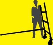
4. Attach a plan brace (black brace) diagonally in a horizontal plane into the base frames as shown.
