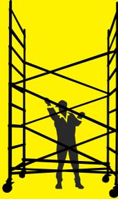
10. Attach a ladder to the inside of the scaffold, through and one (1) metre past the deck to the top transom.
